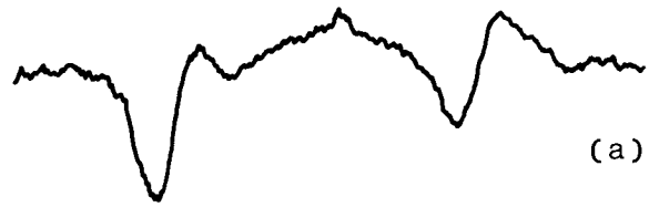
FIG. 5a. — Recorded trace of the ESR absorption line, observed at 1.4 K and 100 GHz for sample M3 ( N_D = 1.9 \times 10^{17} \text{ cm}^{-3} ), in slow passage conditions.
