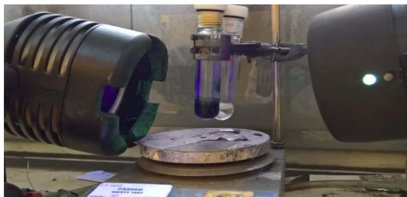
Figure S1 Above is a typical example of reaction performed under UV lamps (365 nm, 100 W x 2) at RT. Left: THF + 17 (0.5 mmol) + KOtBu (2eq). Right: blank reaction THF + 17 (0.5 mmol). Picture taken after 30 min.
