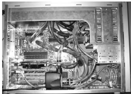
Figure B-1: Localized water cooling applied to personal computer dissipating approximately 100W
