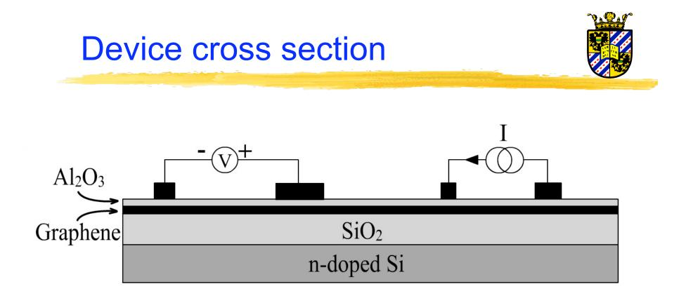
Conductivity mismatch: 1 nm Al<sub>2</sub>O<sub>3</sub> tunnel barrier
