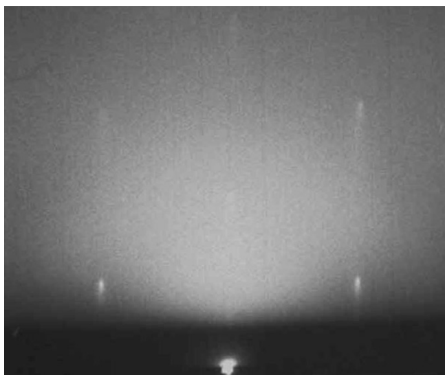
Fig. 2. RHEED pattern of Ta 2 O 5 /Si film.
