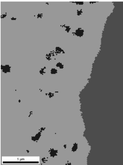
Fig. 5c EDX phase map: TiO 2 particles (black), nickel (light grey), steel (dark grey).
