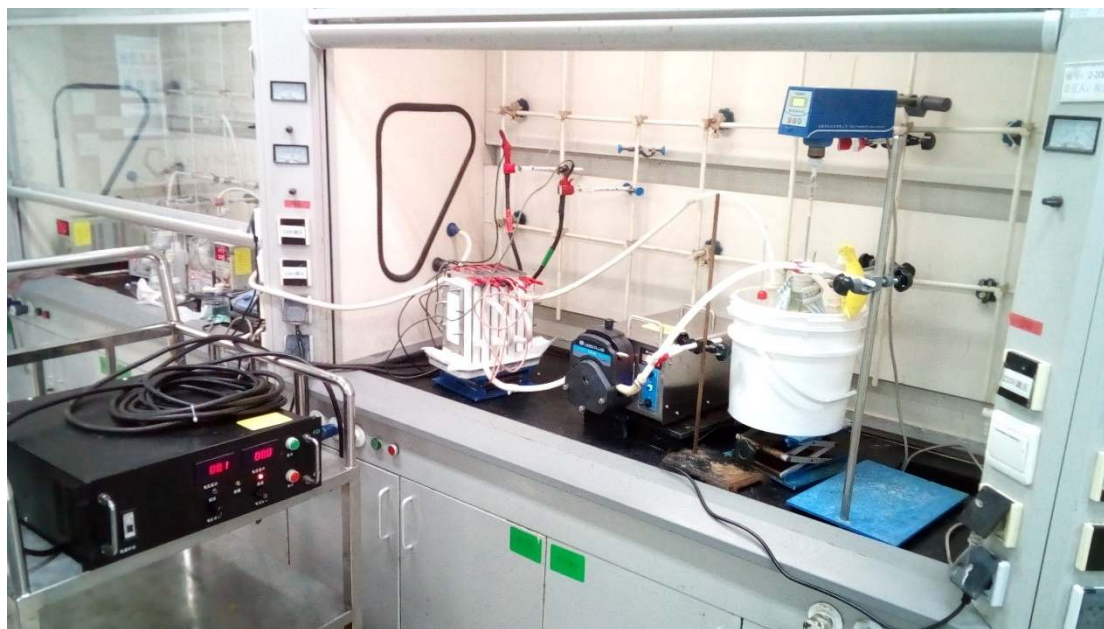
Figure S3. Electrolysis setup in flow cell and local views.
