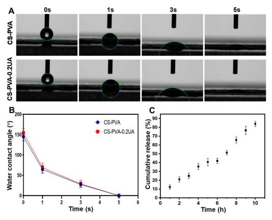
**Figure 4.** (**A**) The actual photographs and (**B**) the corresponding quantitative analysis of dynamic water contact angle of CS-PVA and CS-PVA-0.2UA nanofiber mats (n = 3). (**C**) In vitro accumulated release rates of UA in the CS-PVA-0.2UA nanofiber mat (n = 3).
