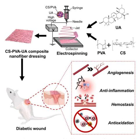
**Figure 1.** Schematic representation of the fabrication process of CS-PVS-UA nanofiber mats and their application as novel wound dressings with multiple functions including hemostasis, antiinflammation, antioxidation, and pro-angiogenesis for the treatment of diabetic wounds.
