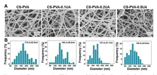
**Figure 2.** (**A**) The representative SEM images and (**B**) the fiber diameter distribution analysis of as-obtained CS-PVA, CS-PVA-0.1UA, CS-PVA-0.2UA, and CS-PVA-0.5UA nanofiber mats using a blend electrospinning strategy.
