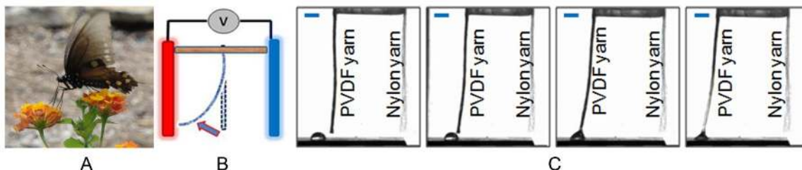
Figure 6.6. (A) Butterfly with a proboscis searching for food. (B) A schematic of yarn manipulation with electric field generated by two vertical electrodes. (C) Artificial proboscis made of PVDF/PEO fibers absorbing a TBP droplet. Two electrodes are positioned from the sides and are not shown here. The solid black fiber on the left is the artificial proboscis; the gray fiber on the right is a nylon yarn. The scale bar is 2 mm.
