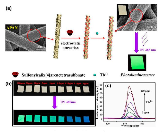
**Figure 5.** Electrospun-NFs-based chemosensors for water pollutant. (**a**) Preparation procedure and photoluminescent behavior of sulfonylcalix[4]arene-functionalized APAN nanofibrous for the adsorptive removal Tb<sup>3+</sup> ions. (**b**) Photographs of NFs after immersing into Tb<sup>3+</sup> aqueous solutions (0–100 ppm). (**c**) Fluorescence spectra of NFs (reproduced with permission from [173], copyright © 2018, Royal Society of Chemistry).
