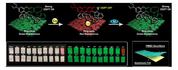
**Figure 7.** Schematic illustration of a ratiometric fluorescent sensing platform that uses a probedoped PMMA material for the specific and visual detection of  $Cu^{2+}$  and ATP sequentially, with photographs of the nanofibers exposed to different metal ions that confirm the selectivity of the platform (reproduced with permission from [182], copyright © 2020, Elsevier).
