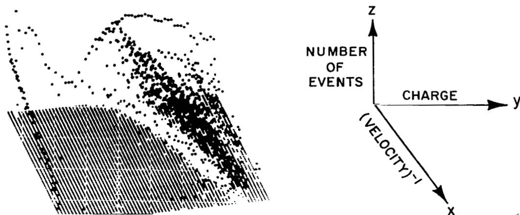
Figure 5.- Output of multiparameter pulse-height analyzer showing charge-velocity spectrum
