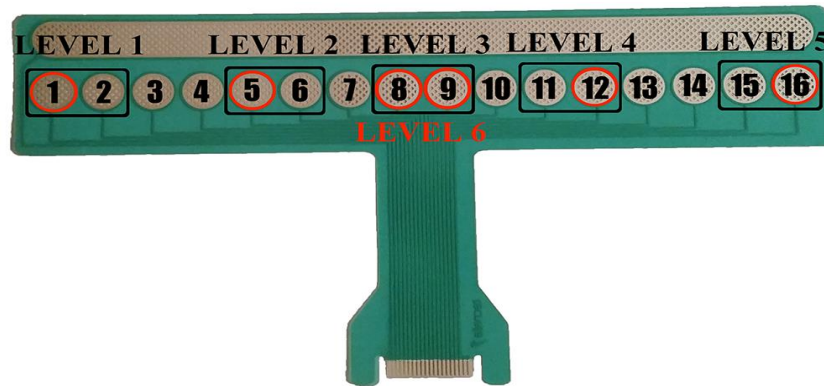
Fig 2. The stimulation array electrode, consists of 16 circular cathodes and a single anode stretching alongside, used for electrotactile feedback. The pads used for feedback mapping are marked with black rectangles (Levels 1 – 5) and red circles (Level 6).
