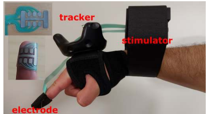
Fig. 2. Experimental apparatus. The electrical stimulator is attached to the forearm and the electrode is placed in contact with the finger pad. The two insets represent detailed views of the electrode. The user’s hand is tracked by a HTC Vive Tracker.
