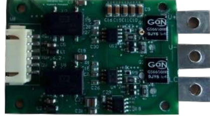
Fig. 22. The implemented GaN based half-bridge inverter module
