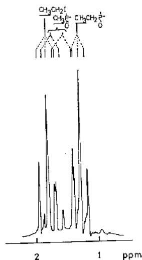
Figure 2. NMR spectrum of the reaction products from ethyl iodide and 2-methoxy-1,3,2-dioxaphospholane in P-CH 3 region: [ethyl iodide] 0 = 2.51 M; [2-methoxy-1,3,2-dioxaphospholane] 0 = 2.91 M.
