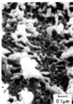
Fig. 1. Scanning electron microscope image of the surface topography of a commercial ammonia synthesis catalyst [5].
