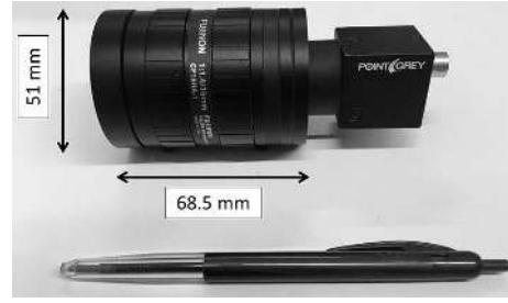
Fig. 4. The camera and lens used in this experiment. The field of view is about 37-degree width. The focal length and f-number were fixed during the experiment.
