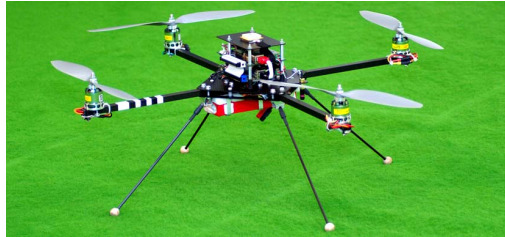
Fig. 3. The I4Copter quadrotor helicopter; specifically designed with a redundant set of sensors.
