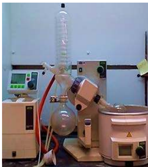
Figure 14. Evaporation of solvent with a rotary evaporator.
