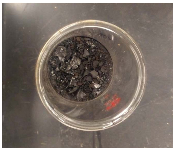
Figure 12. Separation of asphaltene.
