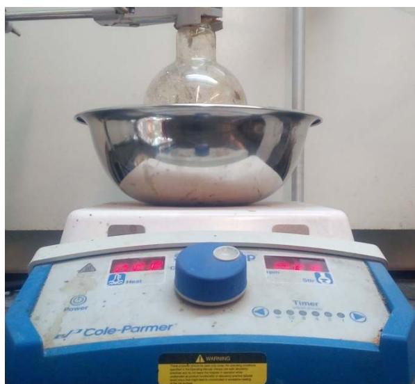
Figure 11. Dissolving asphalt on n-heptane.
