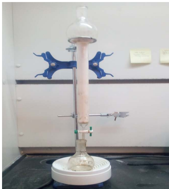
Figure 13. Separation of aromatics, resins, and asphaltenes.
