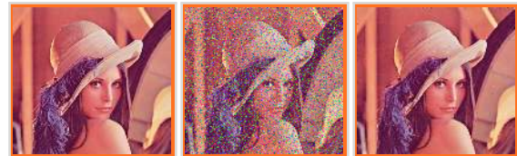
(a) clean ‘lenna’ (b) corrupted ‘lenna’ (c) recovered ‘lenna’ Figure 9: Colored image denoising problems.
