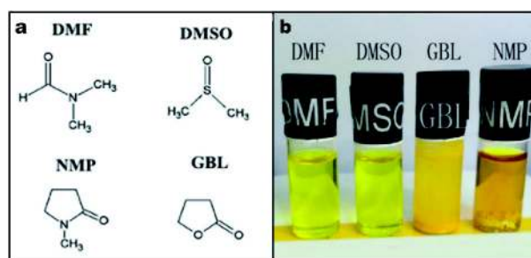
Figure 1 (a) Molecular arrangement of DMF, GBL, NMP, and DMSO. (b) The solubility of the \text{PbI}_2 precursor at 75°C in DMF, DMSO, GBL, and NMP. Both DMSO and DMF: liquefied; GBL: colloidal suspension; NMP: partially liquefied. Reprinted with permission from Ref. [30], Copyright 2014, the Royal Society of Chemistry.
