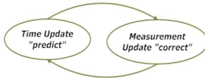
Fig. 1. Kalman filter cycle
