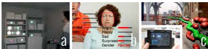
Fig. 7. Examples of embedded visualizations which use projection and video see-through to visualize data about (a) physical inventories [41], (b) faces 2 , and (c) air quality [49] on top of their physical referents.
