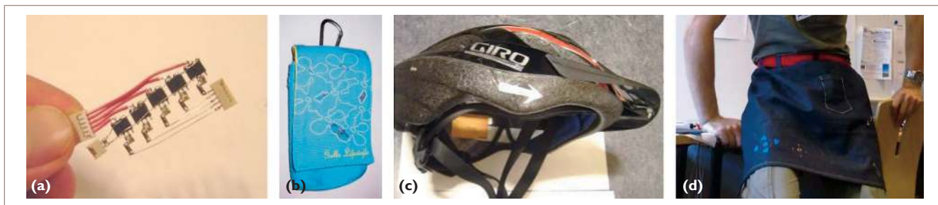
Figure 2. Touch sensors in clothing and accessories. We put (a) flexibly soldered sets of touch sensors (QProx QT110) into several device prototypes, including a (b) phone bag, (c) bicycle helmet, (d) and piece of clothing with different designs for touch areas.
