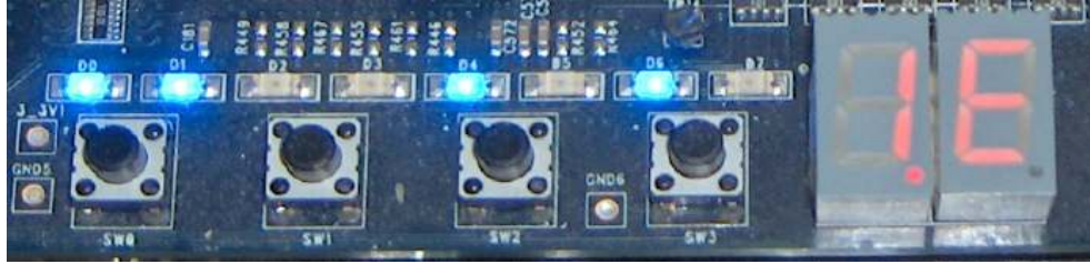
Figure 3.9: LED and seven segment monitoring
