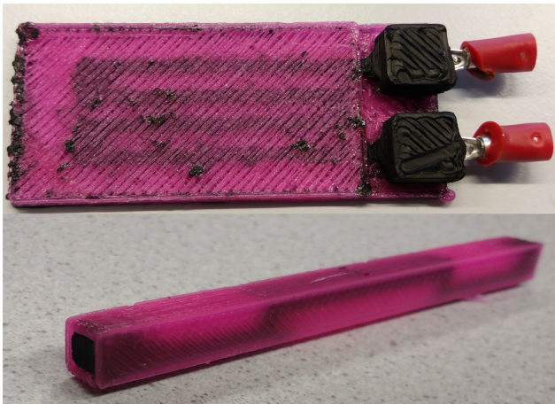
Figure 14. 3-D printed integrated strain sensors.
