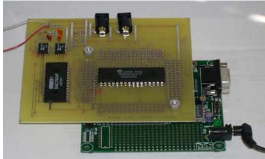
Figure 2 – A Wireless Active Sensing Unit
