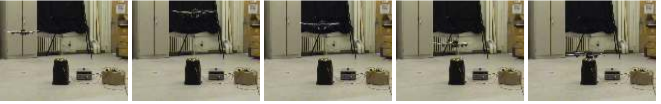
Fig.6: Automated landing and recharge using the RAVEN at MIT [10]
