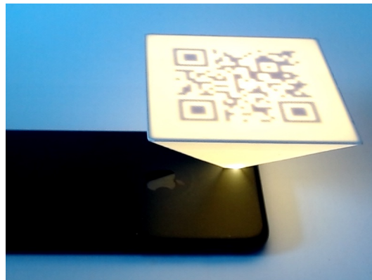
Figure 3. Hidden QR code at the base of the part.
