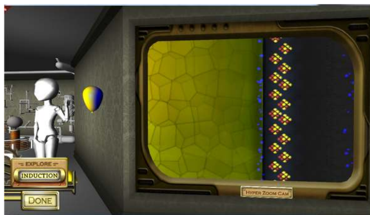
Fig. 5 The negative electrons on the balloon push the negative electrons on the wall deeper into the wall, so the balloon can bond momentarily with the slightly more positive wall surface
