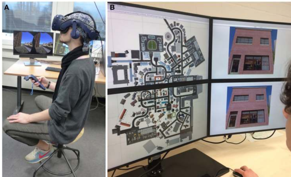
FIGURE 3 | Experimental setup: the VR experimental setup includes the HTC Vive, controller, and swivel chair (A). The experimental design with the interactive map is shown in (B) (written informed consent was obtained from the individuals for the publication of these images).
