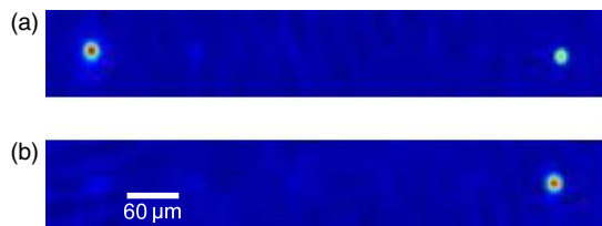
FIG. 2 (color online). (a) Absorption image of the cloud after the application of a 30\hbar k SB-LMT beam splitter. The beam splitter consists of five sequential 6\hbar k pulses (one \pi/2 pulse, four \pi pulses). The image is taken after 4 ms time-of-flight from the application of the first pulse, corresponding to a wave packet separation of 600 \mu\text{m} . The faint spots between the two main wave packets arise from pulse inefficiency due to imperfections. (b) Image of the cloud after the application of five consecutive 6\hbar k \pi pulses, effectively forming a 30\hbar k SB-LMT \pi pulse. Each 6\hbar k \pi pulse has an efficiency of 94%, corresponding to a total efficiency of \sim 73\% for the five pulse sequence. False color red corresponds to a higher atom density [33]. The images in this figure have been rotated by 90^\circ .
