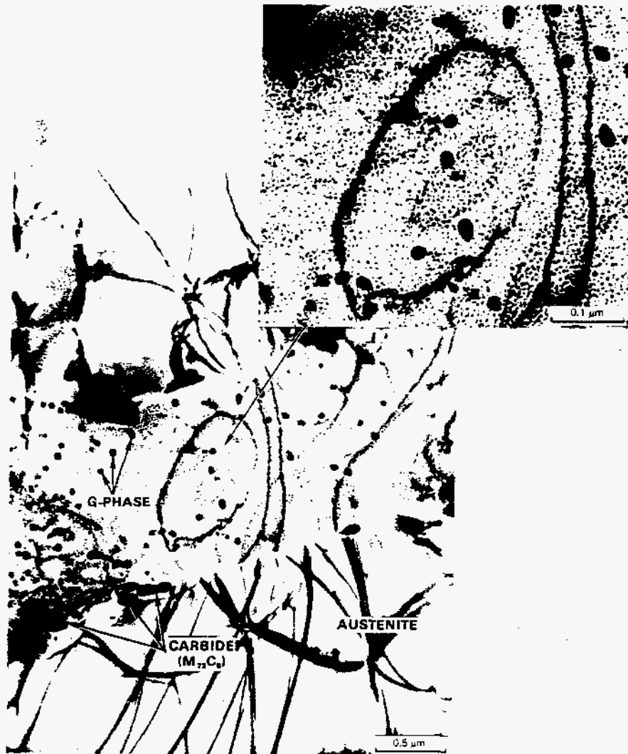
Figure 4. Electron micrograph of decomposed ferrite in a weld aged at 475° C for 5000 hr. The electron micrograph shows the G-phase, M_{23}C_6 carbides, and the mottled nature of the spinodally decomposed ferrite into \alpha and \alpha' phases.
