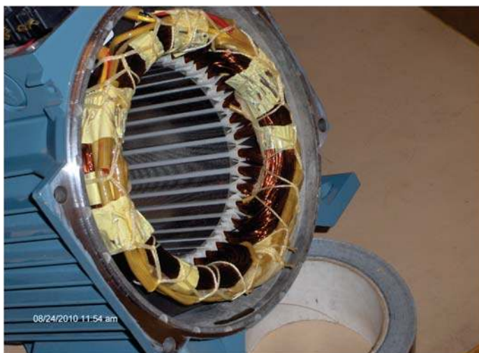
Figure 2.1: A photo of induction machine stator showing Integral Slot, Single Layer Winding of q=3 (36 slots, 3 phases & 4 poles) as well as the End Turns arrangement
