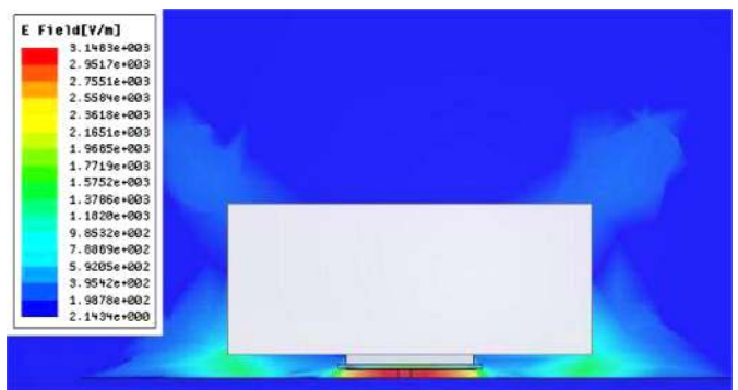
Fig. 3. The side view of the radiation energy flow observed from Intel P4 CPU heat sink simulation model with finite ground plane. (Color version available online at http://ieeexplore.ieee.org .)
