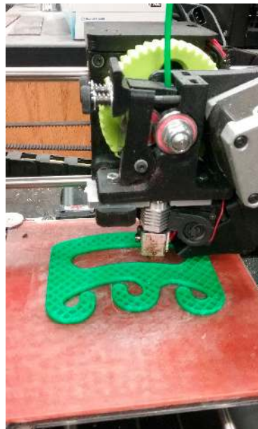
Figure 1. Lulzbot Mini mid-print using poly lactic acid and Cura Quick Print settings.
