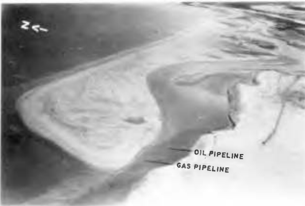
Figure 6. Undermined Pipelines Date: 03/02/88 Hour: 10:24 W.L.= +0.7m
