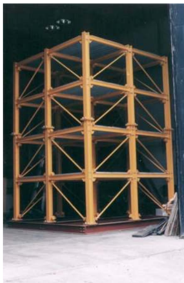
Fig. 4 IASC-ASCE benchmark structure (Photo courtesy Prof. Carlos Ventura, UBC)
