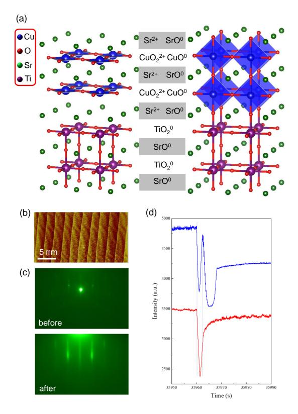
FIG. 1. (color online) (a) Schematic plots of the planar-type (left) and the chain-type (right) tetragonal SCO on TiO<sub>2</sub>-terminated SrTiO<sub>3</sub> substrates. (b) Surface morphology of TiO<sub>2</sub>-terminated SrTiO<sub>3</sub> substrates characterized by an atomic-force microscope.
