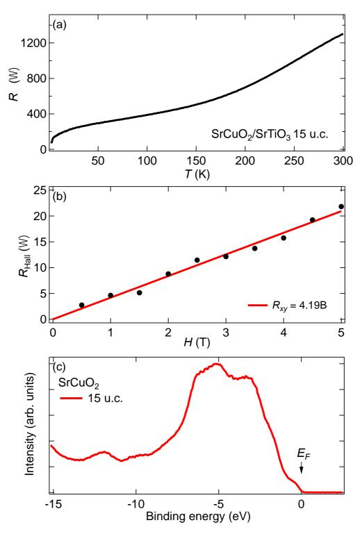
FIG. 2. (color online) (a) Sheet resistance  $R_{\Box}(T)$ , (b) Hall resistance, and (c) the valence band HAXPES spectrum of a 15 u.c. SCO/STO (For discussions, see SM). The Hall and HAXPES measurements were performed at 300 K.
