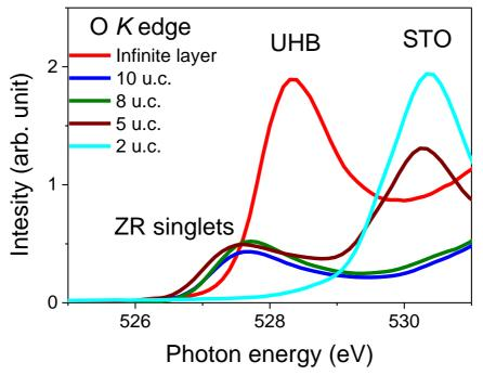
Fig. S6 **O** *K*-edge XAS of SCO/STO with various SCO thickness. The presence of Zhang-Rice (ZR) singlet in SCO with thickness larger than 5 u.c. generally coincidences with a significant electrical conductivity (see Figs. S1 and S3). The feature near 530.3 eV, clearly seen in 2 u.c. and 5 u.c. samples, is attributed to the STO substrate.
