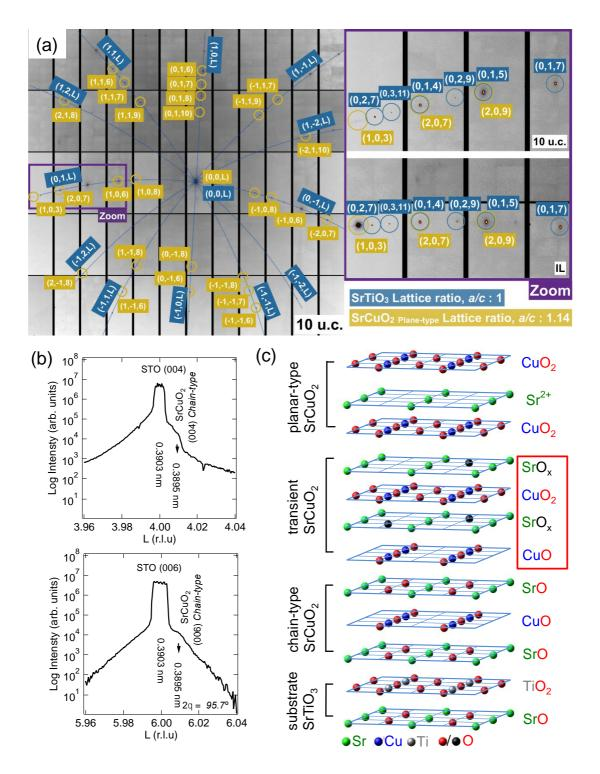
FIG. 4. (color online) (a) White-beam Laue diffraction pattern of a 10 u.c. SCO/STO sample. The diffraction peaks from STO substrate and the planar-type SCO are marked in steel blue and gold colors, respectively. The zoom in images (purple box) show the diffraction patterns of a 10 u.c. SCO/STO and an IL SCO. The (103) lattice plane of planar-type SCO can be clearly seen in the Laue patterns because of the
