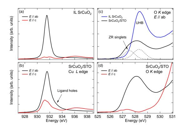
FIG. 3. (color online) Polarization dependence of Cu *L*-edge XAS spectra of (a) IL SCO and (b) the 15 u.c. SCO/STO. Black and red lines are spectra with E//ab and E//c, respectively. (c) O *K*-edge XAS spectra of IL SCO and 15 u.c. SCO/STO; (d) Polarization dependence of O *K*-edge XAS spectra of 15 u.c. SCO/STO. The dashed lines in (c) denote the respective components for ZR singlets and UHB for SCO/STO.
