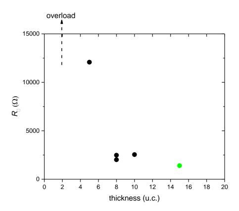
Fig. S4 Thickness dependence of  $R_{\Box}$  at 300K. The black solid circles are the  $R_{\Box}$  values of one batch of SCO/STO ultrathin films with thickness ranging from 2 u.c. to 10 u.c.  $R_{\Box}$  of 2 u.c. sample is too large to be measured accurately even at the room temperature. The green solid circle denotes the  $R_{\Box}$  value of the metallic SCO/STO (15 u.c.) shown in the manuscript.
