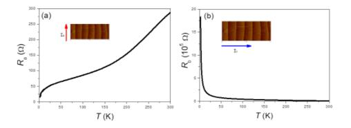
Fig. S5 Anisotropic  $R_{\Box}(T)$  of the metallic SCO/STO. Metallic SCO/STO samples similar to the one in Fig. 2(a) in the manuscript all show a large anisotropy with respect to the direction of applied current ( $I_b$ ). We believe this anisotropy is due to steps on the substrates as revealed in the AFM images (inset). When the direction of applied current  $I_b$  is nearly perpendicular to the steps (right panel), these samples
