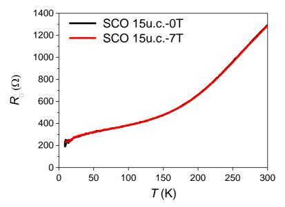
Fig. S2 Absence of Magnetoresistance. Sheet resistance  $R_{\Box}(T)$  of a 15 u.c. SCO/STO measured at zero field (black line) and 7 T field (red line). There is no appreciable magnetoresistance in this sample.
