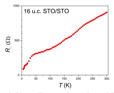
Fig. S1 **Reproducible metallic state.** Sheet resistance  $R_{\Box}(T)$  of another SrCuO<sub>2</sub>/SrTiO<sub>3</sub> (SCO/STO, 16 u.c.) sample showing the metallic behavior. This sample was measured in a different setup (Quantum Design<sup>©</sup> electrical transport Option, ETO) compared to the ordinary 4-probe DC method used in Fig. 2 in the manuscript. Using two separate measurement setups to avoid systematic error, the metallic behavior was independently verified.
