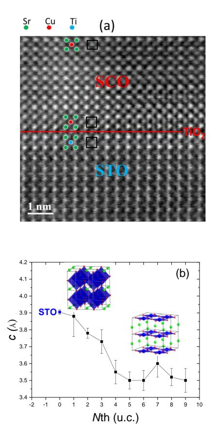
Fig. S7 **STEM image and the measured** *c***-axis lattice constant.** The scanning transmission electron microscopy (STEM) images were taken using JEOL ARM200F equipped with a spherical aberration (Cs) corrector at 200 kV accelerating voltage.
