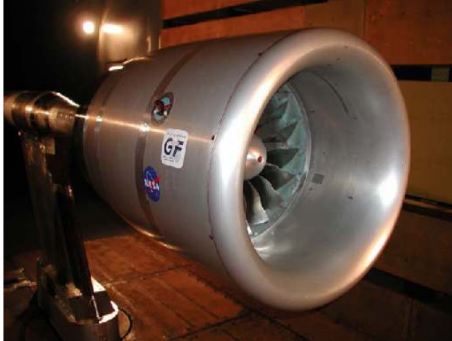
Figure 5.—NASA/P&W 22-in. scale model Geared Turbofan (GTF) rig installed in the NASA 9- by 15-ft Low Speed Acoustic Wind Tunnel. Test results confirmed the acoustic benefits of ultra-high bypass ratio cycles.
