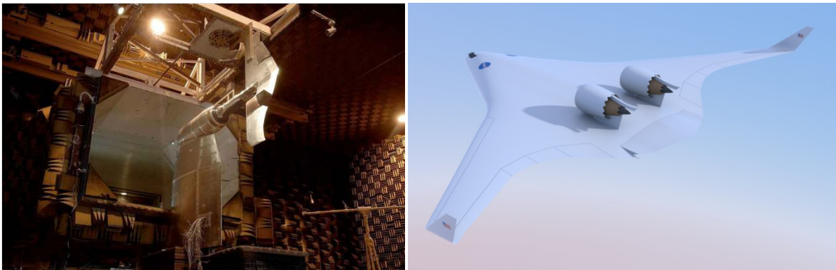
Figure 13.—NASA/Boeing propulsion aeroacoustics tests were conducted in Boeing's Low Speed Aeroacoustic Facility shown on the left. In the middle of the picture is the simulated nozzle just to the left of the Blended Wing Body planform suspended vertically from the ceiling. On the right, is an artist's rendering of the quietest configuration studied in References 4 and 5. Note the location of the nozzles (fan and core) both of which are located well upstream of the BWB trailing edge to shield the noise from reaching the observer below. The design of the chevrons and pylons (in keel and crown positions) were optimized for noise reduction.
