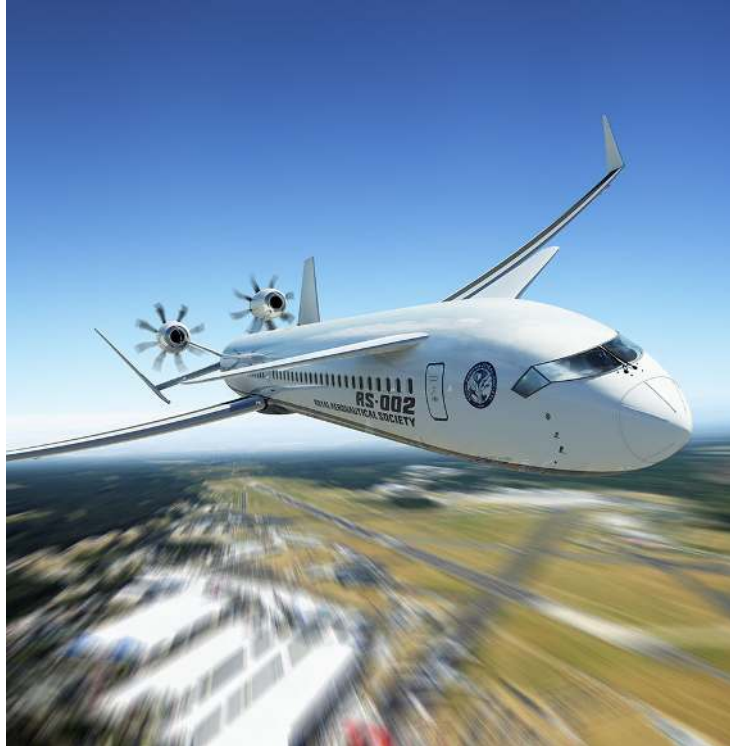
Figure 15.—The type of empennage shielded open rotor engine installation analyzed in the study described in Reference 32. The U-tail is providing significant shielding below and to the side of the engines.
