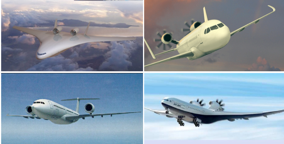
Figure 12.—Four novel engine/airframe integration concepts with the potential for significant shielding of engine noise by the airframe.
