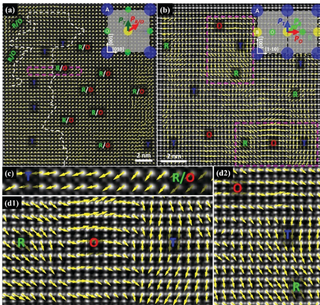
Fig. 9 Local symmetry and polarization mapping inside nanodomains of KNNS–BNKZ–AS–Fe ceramics. Atomically resolved STEM HAADF images along (a) \langle 100 \rangle and (b) \langle 110 \rangle zone axes. The corresponding insets show the schematic project of the ABO_3 unit cell along \langle 100 \rangle and \langle 110 \rangle zone axes. When viewing the unit along the \langle 100 \rangle zone axis, the T phase exhibits the polarization vector along (001)_{pc} , while both R and O phases display similar polarization vectors along (110)_{pc} . When viewing the unit along the \langle 110 \rangle zone axis, the T phase exhibits the polarization vector along (001)_{pc} , the O phase displays the polarization vector along (110)_{pc} , and the R phase displays the polarization vector along (111)_{pc} . (c) Enlarged image of the marked area in (a) showing the transition of polarization vectors from T to O/R. (d1 and d2) Enlarged images of the marked areas in (b) showing the transition of polarization vectors from R to O to T. (a–d2) Reproduced from ref. 24 with permission from the American Chemical Society, Copyright 2019.
