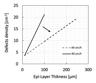
**Figure 6.** Electrical defect density vs. epi layer thickness for two different high-growth-rate processes. A considerable improvement in the defects' density has been observed at the lower growth rate.
