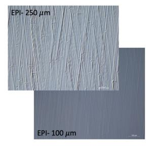
**Figure 7.** Optical microscope images of two different epitaxial layer thicknesses. It is possible to observe an increase in the roughness, increasing the thickness.
