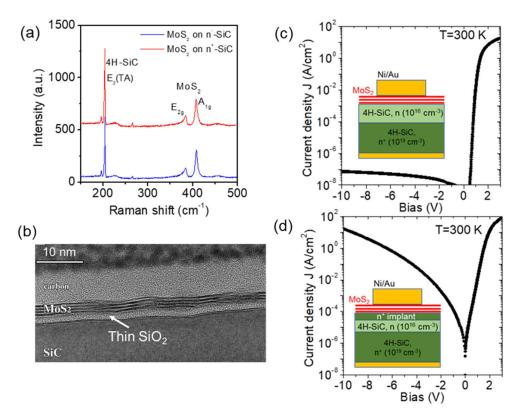
Figure 10. (a) Raman spectra of PLD-grown MoS2 on n- and n+-doped 4H-SiC. (b) Cross-sectional TEM showing conformal coverage of 3L-MoS2 on the  $4^{\circ}$ -off 4H-SiC surface, with the presence of an ultra-thin SiO<sub>2</sub> interfacial layer. (c) Current–voltage characteristics, measured at T = 300 K, of MoS<sub>2</sub> heterojunction diodes with an n- 4H-SiC epilayer and (d) n+-implanted 4H-SiC. Image adapted from Ref. [125].
