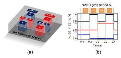
**Figure 5.** (a) Schematic structure of a SiC CJFET and (b) characteristics of a NAND gate at 350  $^{\circ}$ C fabricated with SiC CJFET [61].
