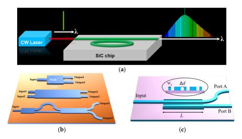
**Figure 13.** Schematic of basic building blocks to construct optical chips: (a) An optical frequency comb light source; (b)  $1 \times 2$  multimode interference (MMI),  $2 \times 2$  MMI, and Mach-Zehnder interference (MZI) splitter; and (c) polarization beam splitter with vertical-dual-slot waveguides.
