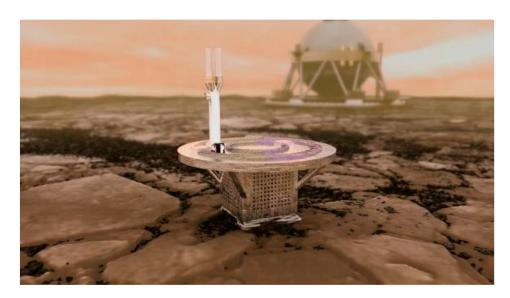
**Figure 2.** Concept of ~10 kg LLISSE lander conducting a 60-day mission on Venus enabled by SiC electronics operation unprotected from the 460  $^{\circ}$ C 9.3 MPa surface environmental conditions. In the background is a protected-electronics lander design weighing over 500 kg whose mission duration is less than 1 day [40].
