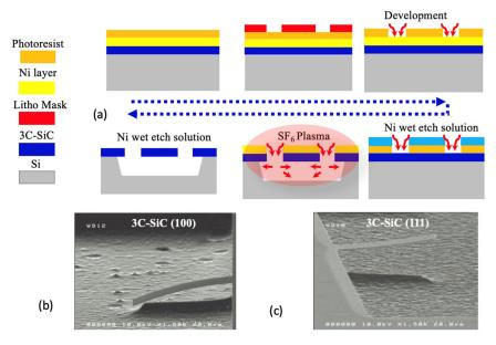
**Figure 11.** (a) Cross-sectional schematics of the 3C-SiC micromachining process and SEM images of clamped beams obtained by this process dependent on orientations (b) 3C-SiC (100) and (c) 3C-SiC(111) bending, respectively, downward and upward (issue from [143]).
