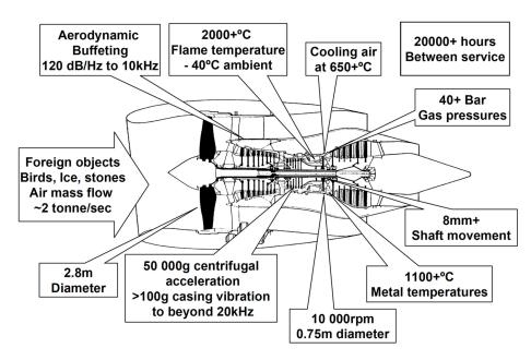
**Figure 1.** Environmental challenges of the jet engine environment [33].
