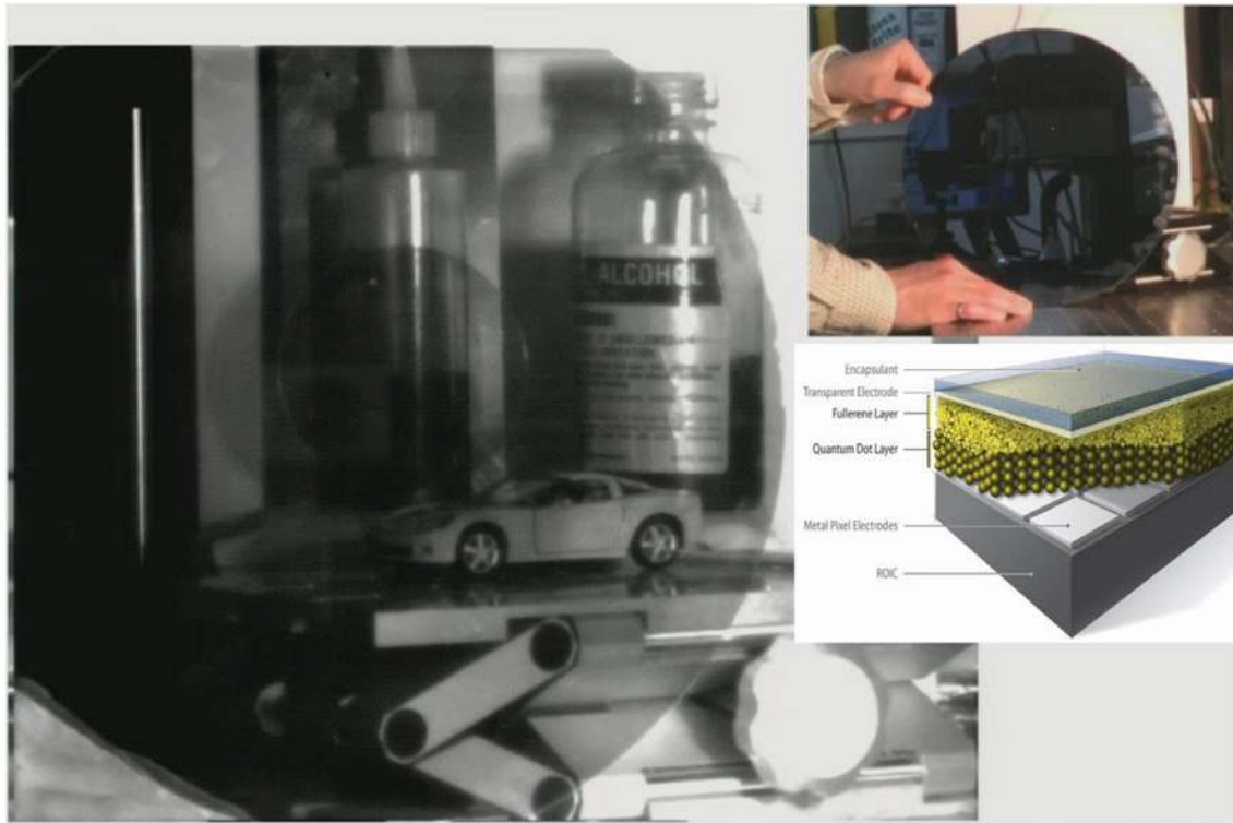
Figure 9: An image from the PbS CQD-based focal plane array (FPA) camera operating in the SWIR band. The CQD-based camera can see through a silicon wafer. The first inset shows the image taken using a normal visible camera. Second inset image is the PbS CQD-based focal plane array (FPA) structure [162].
