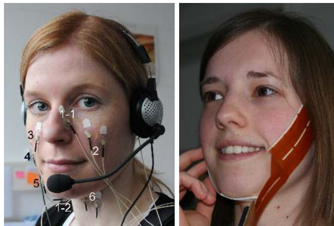
Figure 4.1 – The single-electrodes recording setup (left) and electrode-array recording setup (right).
