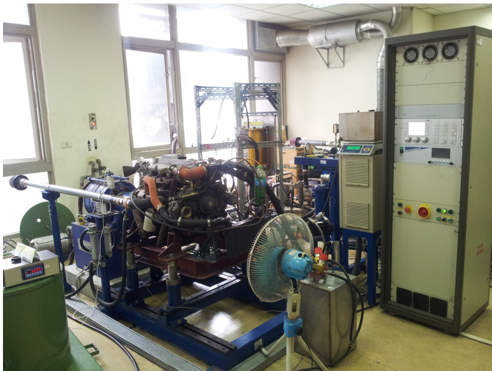
Fig. 1. Diesel engine and control system.
