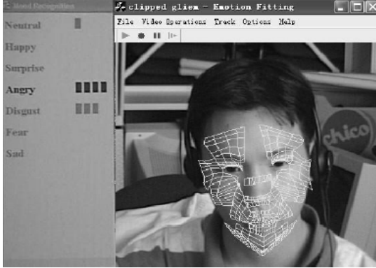
Figure 1. A snap shot of our facial expression recognition system. On the right side is a wireframe model overlaid on a face being tracked. On the left side the correct expression, Angry, is detected.
