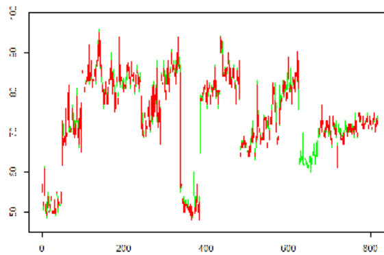
Figure 2. HR signal gathered using the Empatica E4 (red line) and Biopac MP150 (green line). X-axis corresponding to the full dataset. Y-axis corresponding to the Heart Rate.
