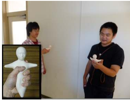
Fig. 1. Elfoid: cellular phone-type teleoperated android
