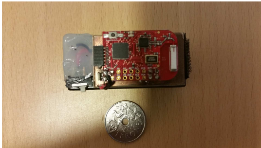
Fig. 3. Practical sensor node for path loss measurements consists of a radio transceiver, antenna, microcontroller, microSD memory card and battery. Shown together with Norwegian one krone.
