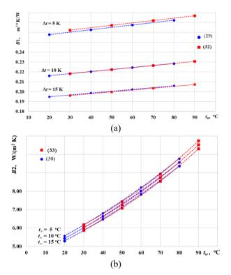
**Figure 3.** Values of *B*1 calculated from Eqns. (29) and (32) for  $\Delta t$ =5, 10 and 15 K as a function of the heating surface temperature varying in the range  $t_{\rm w}$ =20 – 90°C (a) compared with values of *B*2 calculated from Eqns. (30) and (33) for  $t_{\infty}$ =5, 10 and 15 K ( $\Delta t$ = $t_{\rm w}$  –  $t_{\infty}$ ) as a function of the heating surface temperature varying in the range  $t_{\rm w}$ =20 – 90°C (b)
