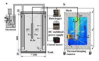
**Figure 7.** Diagram of the experimental apparatus for examining: a) free convective heat transfer in water, using the balance method and an isothermal vertical plate, b) total convective and radiative heat transfer in air, obtained by the use of balance method, and the convective only, obtained by the gradient method, with the additional use of IR camera with detection mesh [71]
