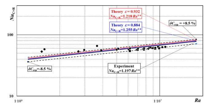
**Figure 8.** The results of the experimental tests, some of which - from Series I (diamonds) and Series II (squares) - are included in Table 3, and the remaining (Series III) experimental points (shown by dots) are not shown in Table 3. The black line shows the approximation of all the experimental results (41). The theoretical solution obtained for  $\varepsilon$ =0.884 is shown by the blue line, and the one for  $\varepsilon$ =0.932 by the red line
