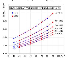
**Figure 4.** Comparison of values of *B*1•*B*2 calculated from Eqns. (34) (blue circles) and (35) (red squares). Eq. (36), shown in the box, is the result of the approximation of the curves obtained using Eq. (34)
